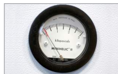
Differential pressure indicator for filter monitoring
